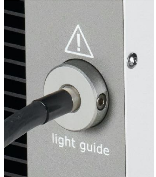
Figure 2. 3 mm diameter liquid light guide inserted in front panel light output port.
