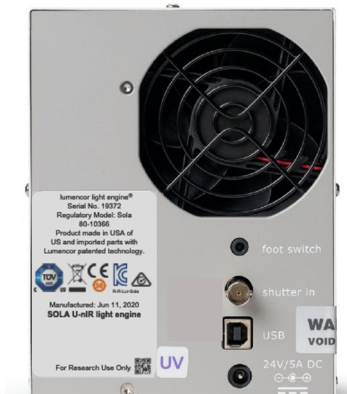
Figure 1. Model and serial number identification label on the SOLA U-nIR light engine rear panel.
