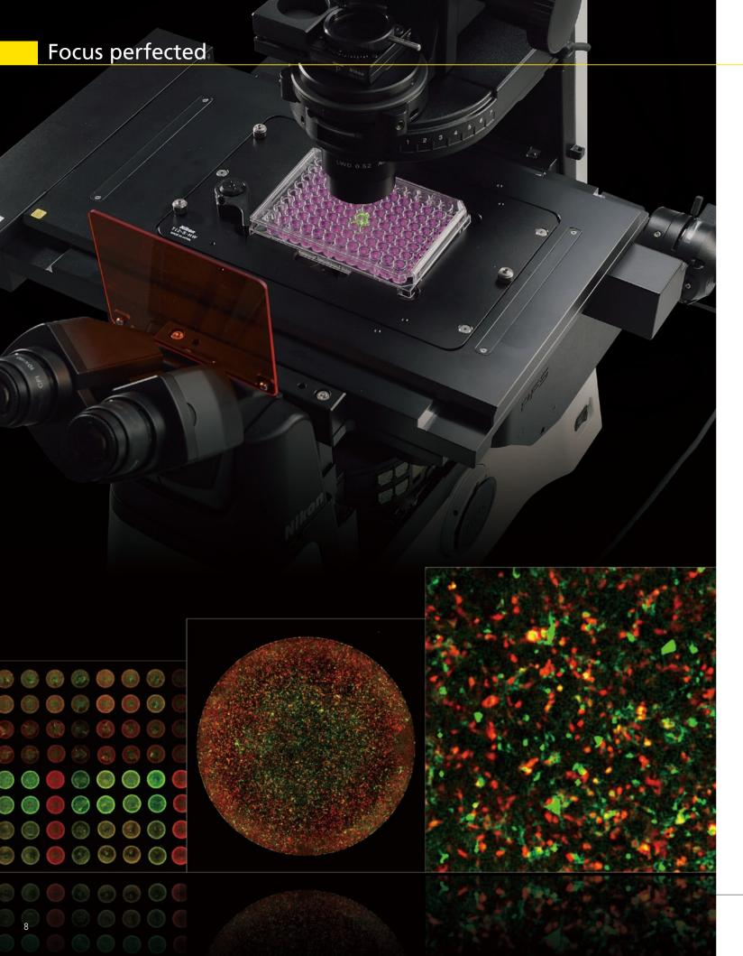
Even the slightest change in temperature and vibrations in the imaging environment can greatly impact focus stability. The Ti2 eliminates focus drift using both static and dynamic measures to enable faithful visualization of the nanoscopic and microscopic world during long time-lapse experiments.
