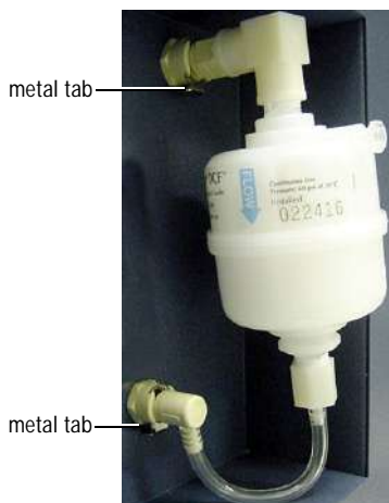
Figure 4-3 Removing a filter
