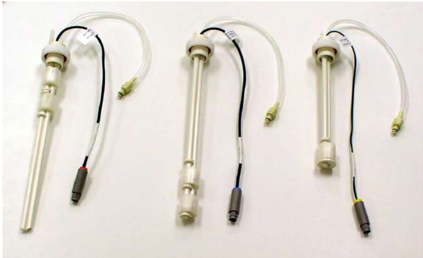
Figure 4-7 Level sensor assemblies
