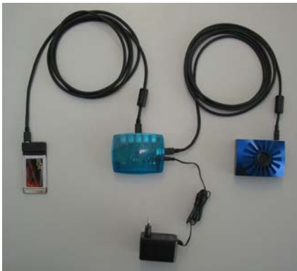
Connecting the AxioCam MR to the FireWire PCCard interface card
