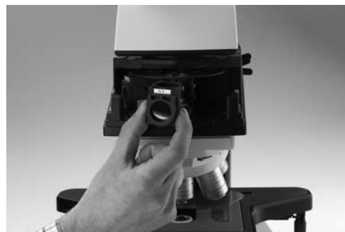
Fig. 25 Mounting the Filter cube
