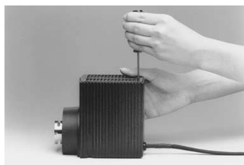
Fig. 14a Lamp housing 107/2 Releasing the fastening screw
