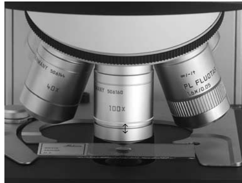
Fig. 55b Immersion objective (locked)
