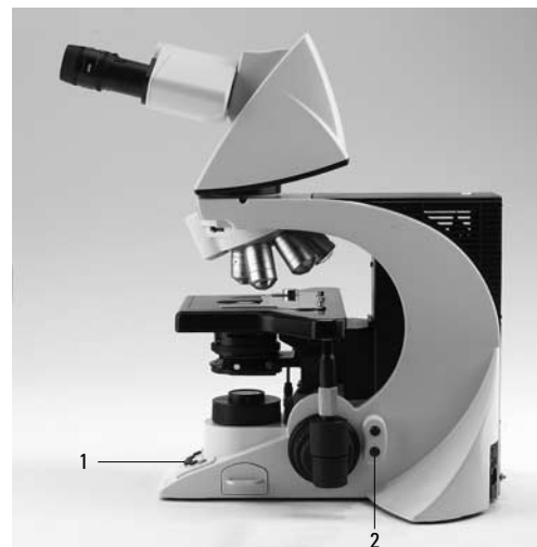
Fig. 56 Leica DM3000 1 Front control panel 2 Lateral function keys
