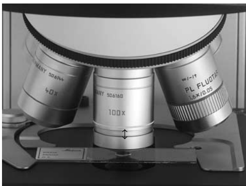
Fig. 55a Immersion objective (released)
