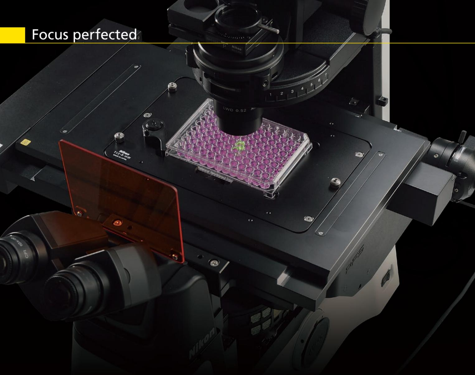
Even the slightest change in temperature and vibrations in the imaging environment can greatly impact focus stability. The Ti2 eliminates focus drift using both static and dynamic measures to enable faithful visualization of the nanoscopic and microscopic world during long time-lapse experiments.
