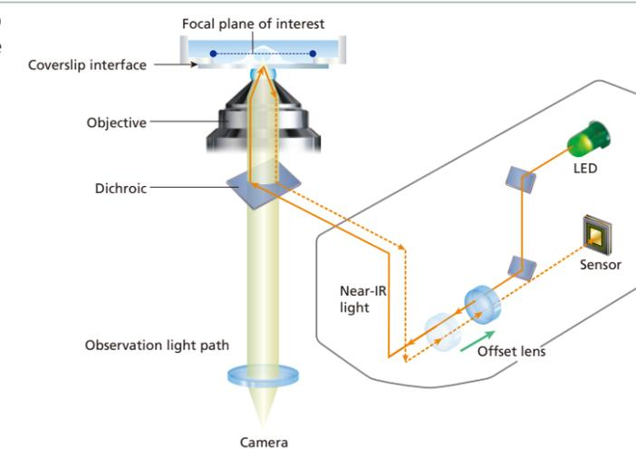
PFS is compatible with a wide range of applications, from routine experiments involving plastic culture dishes to single-molecule imaging and multi-photon imaging. It is also compatible with a wide range of wavelengths, from ultraviolet to infrared, meaning it can be used for multi-photon and optical tweezer applications.
