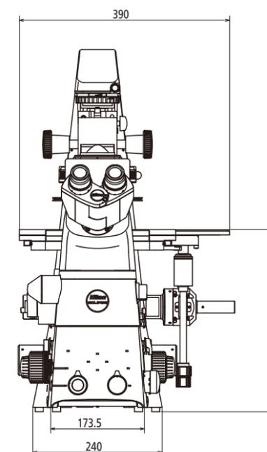
Single layer configuration with an Epi-FL module
